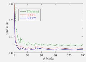
Characteristic zig-zag pattern due to commensurability (or not) of block number of with number of multiprocessors.
